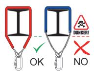
**Protect structure from** wire sling damage
